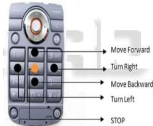
Fig. 8: Functionality of used keypad in Mobile Phone [2]
